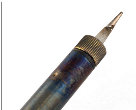
FIGURE 13-5: A soldering iron tip that is in the process of being tinned with solder
